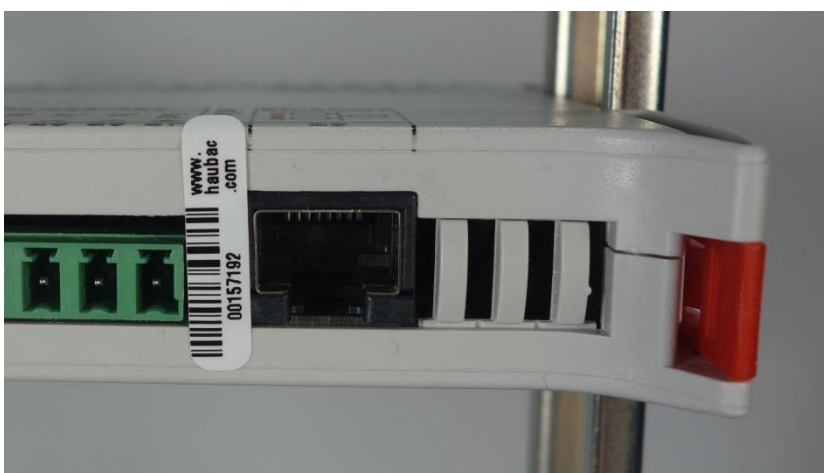
Figure 4 Sealing of DAD14x.y enclosure and calibration jumper
